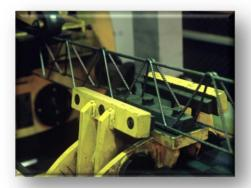
Lattice girders serve some of the best functions in construction support systems, and offer an economical alternative to other support methods for a wide variety of applications.
