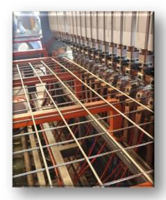
Welded fencing is produced to the highest standards of quality. Thorough testing of wire strength and aperture size is carried out during all stages of manufacturing.
